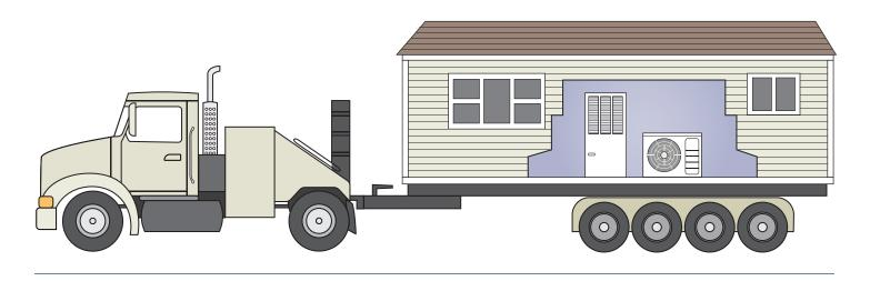
A split-system heat pump consists of three pieces of equipment: the outdoor compressor, the indoor air handler (aka furnace) and the indoor refrigerant coil (which is housed with the air handler). Manufactured home factories currently typically install only the air handler/furnace, leaving the decisions around heat pump equipment sizing and selection to the home retailer or home buyer and their local HVAC contractor.
